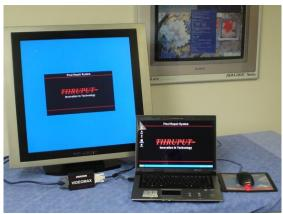
The Videomax I Pixel Repair System is a tool for restoration of normal operation to monitors that have developed a ghosted image, or frozen pixels during their operational life.
